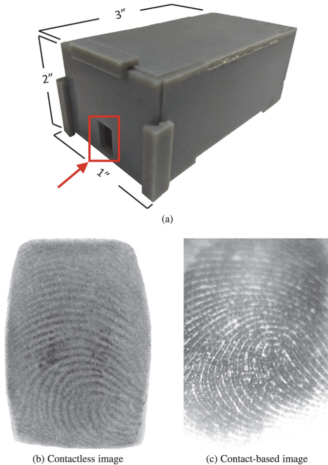
Fig. 6. (a) Prototype of our 1,900 ppi contactless fingerprint reader. During capture, an infant's finger is placed on top of a small, contactless, rectangular opening (annotated in red) on the reader (the size of this opening can be adjusted with different sized slots). A camera captures the infant's fingerprint from behind the rectangular opening. Examples of a processed (segmented, contrast enhanced), contactless infant thumbprint (2 months old) is shown in (b) and the same infant's thumbprint acquired via contact-based fingerprint reader in (c).
